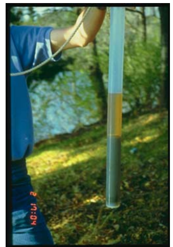
Free product floating on water recovered from a monitoring well
