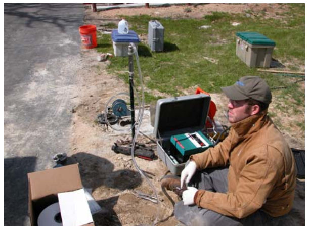
John Hayes supervises a groundwater pumping test
